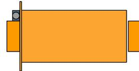
A) (15 pts) As the winch winds in and out, the cable winds on every axial location across the entire length of the drum. Because of this, the location of the 9000 lbs cable tension changes (although you may assume its direction remains nearly constant). Determine the maximum load that could be experienced by the bearings (either on the one on the left or right) and the maximum bending moment that could be experienced by the drum. Show your work.
