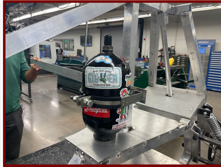
Accumulator mount on Chassis shelf
