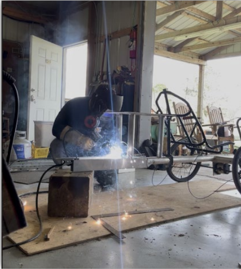
Welding aluminum frame
