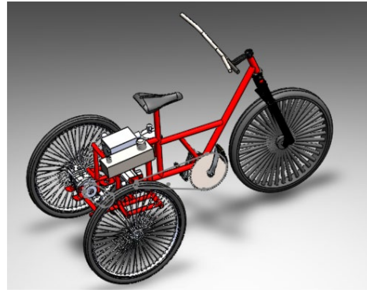
Figure 7: Final Bike Assembly minus hose connections represented in SolidWorks -- Front View
