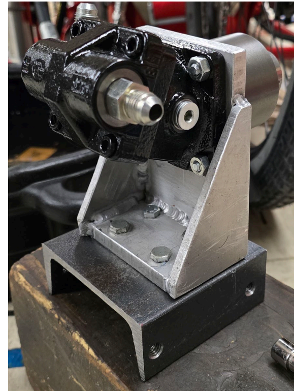
New motor mount uses larger tapped holes instead of slots
