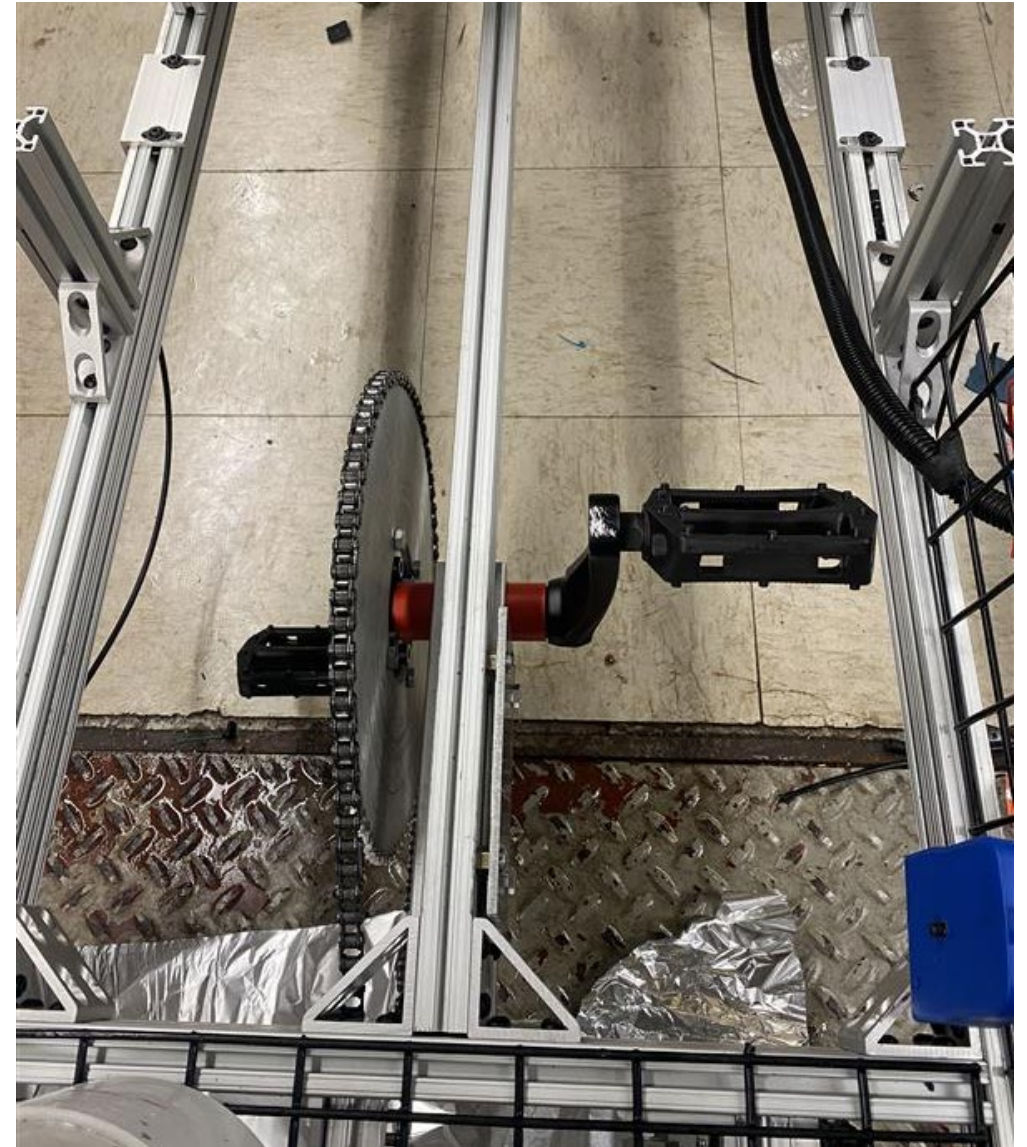
Mounted pedals in 3-point bending rather than a cantilevered beam
