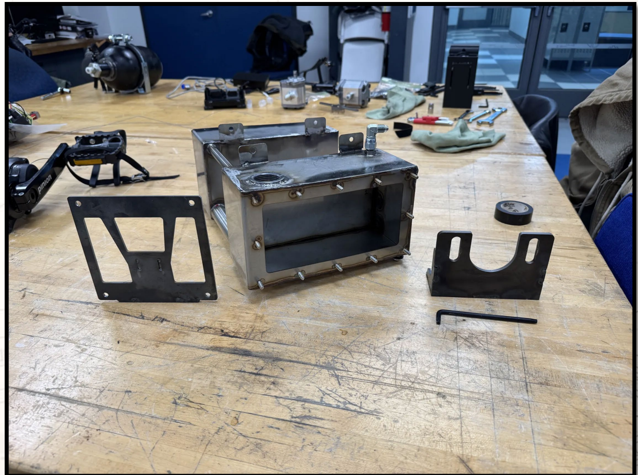
Fig. 20: PLC Mount (left), Hydraulic Reservoir, Regen Pump Mount
