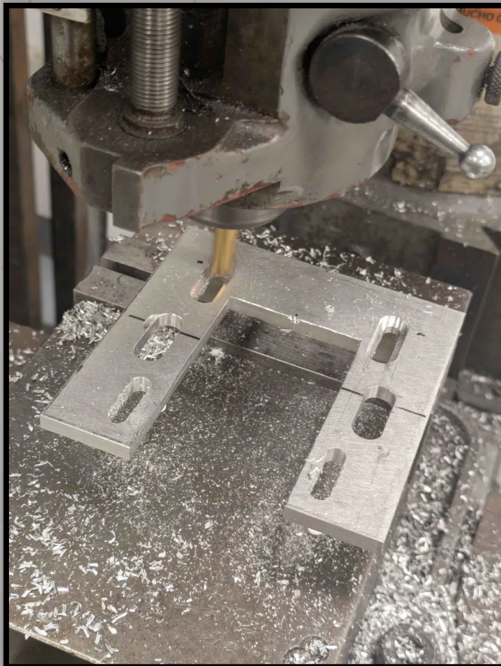
Fig. 19: Hydraulic Motor Mount Fabrication
