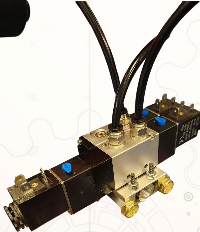
Fig. 28: 3/2 and 5/3 Pneumatic Solenoids on Manifold
