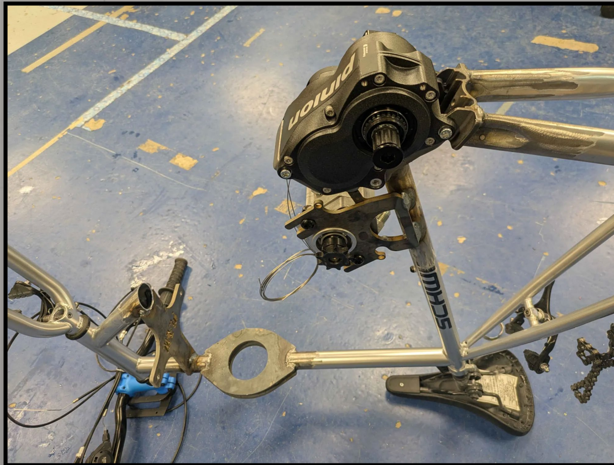
Fig. 17: Frame Accommodations for Accumulator and Pedal Gearbox
