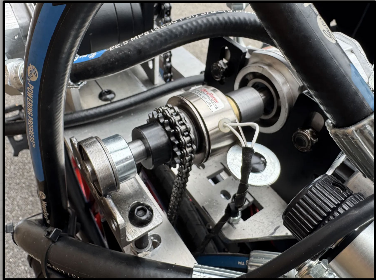
Fig. 12: Clutch Installed on Regen Pump
