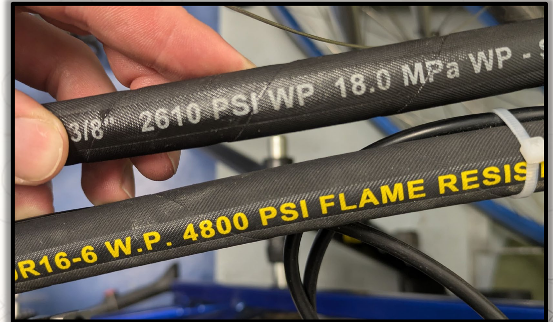
Fig. 8: Hydraulic Hoses from Local Supplier
