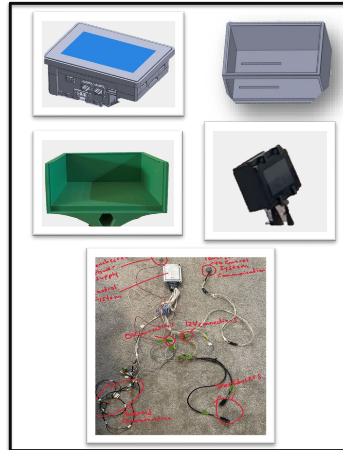
Figure 12. Various Prototypes for HMI Enclosure and Control System Wiring
