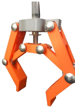
Figure 1. Final assembly of the pneumatic gripper
