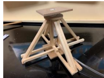
Figure 2. Example deadweight tester built by students
